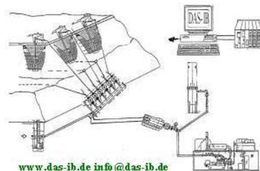
Figure 1 – Landfill gas extraction system (wellheads, manifold station, dewatering system, condensate wells, booster and flare system, gas utilisation facility, telecontrol system)
