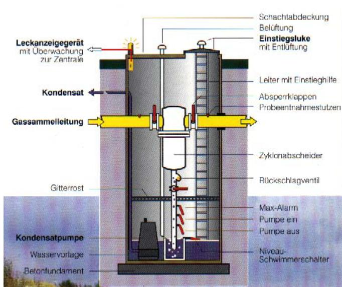
Figure 4– Condensate shaft
