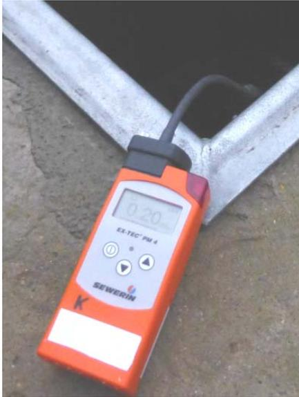
Emission (Vol %) in a manifold station
