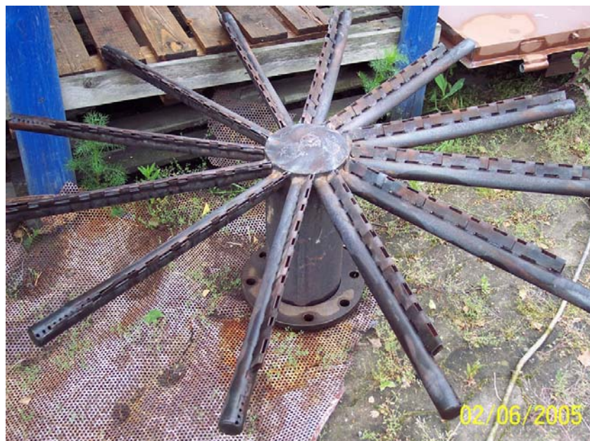
Illustration 1: Example of a burner with damaged burner nozzles (1)
