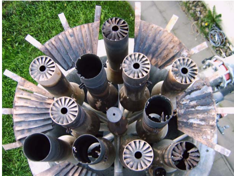
Illustration 1: Example of a burner with damaged burner nozzles (1)
